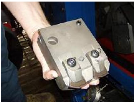
The BT-Z Turning (Peeling) machines use carbide holders that are easily handled by the operator.
