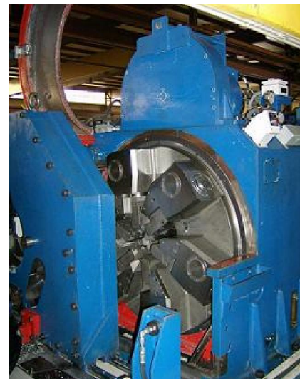
Both the spindle housing "hood" and the entry guide assembly can be retracted to provide optimum accessibility to the carbide holders when changing carbides.
