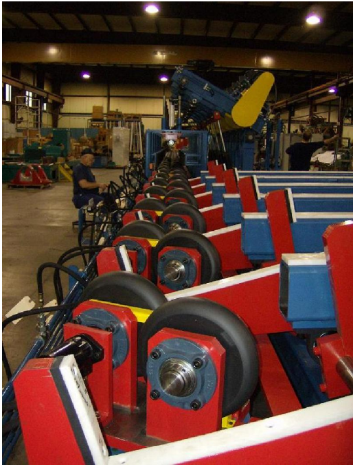
A multi-head polishing line for super finishing peeled shafting bars up to 12" (300mm), prior to plating.
