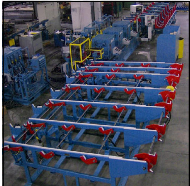
A three head, planetary belt polishing system for titanium bars up to 45mm (1.770") to be installed in-line with a recently commissioned Hetran BT2 bar turner.
