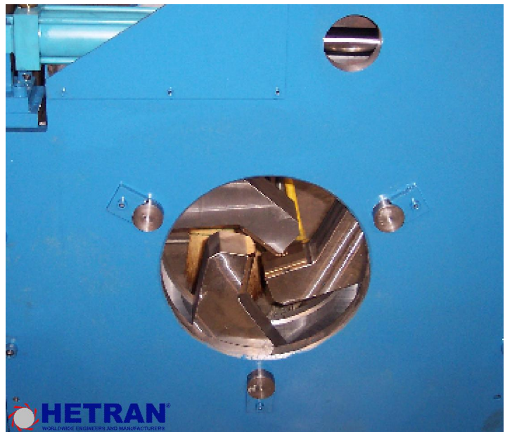
A close up view of Hetran's three jaw entry guide, showing the jaws in the closed position.
