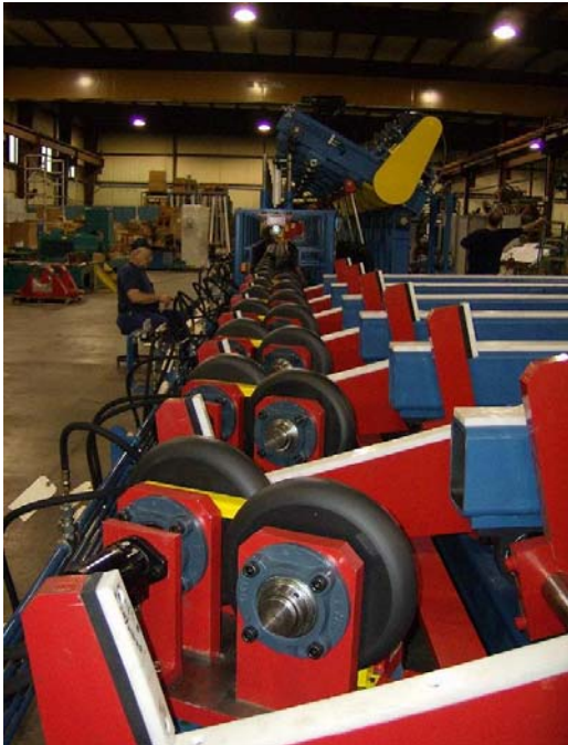
A multi-head polishing line for super finishing peeled shafting bars up to 12" (300 mm), prior to plating.
