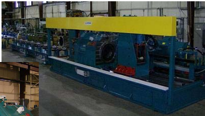
A BT-12 (300 mm) turning (peeling) line for stainless, tool and alloy steels, partially disassembled, and being readied for shipment.
