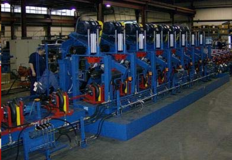
A multi-head polishing line for super finishing peeled shafting bars up to 12" (300 mm), prior to plating.
