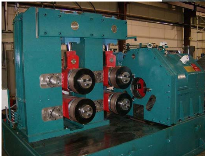
A BT-12 (300 mm) turning (peeling) line for stainless, tool and alloy steels, partially disassembled, and being readied for shipment.
