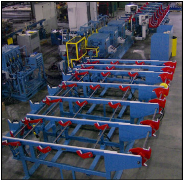
A three head, planetary belt polishing system for titanium bars up to 45mm (1.770") to be installed in-line with a recently commissioned Hetran BT2 bar turner.
