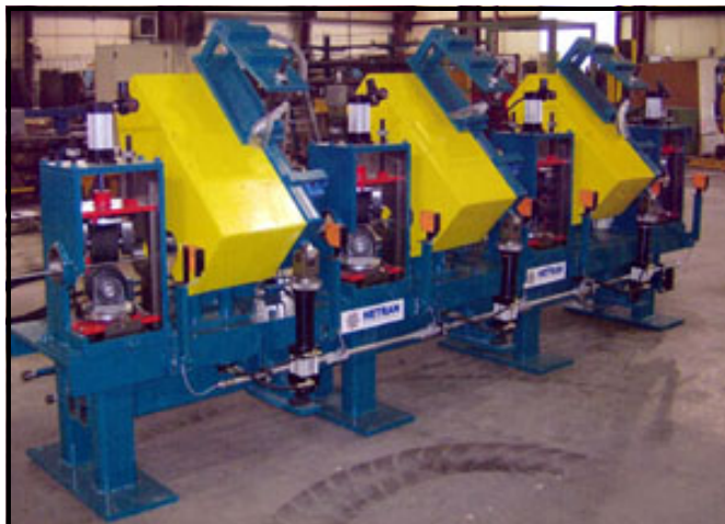
A three head belt polishing system for bearing, tool and alloy steel bars up to 100mm (4") to be installed in-line with an existing Hetran BT4 bar turner and burnisher.
