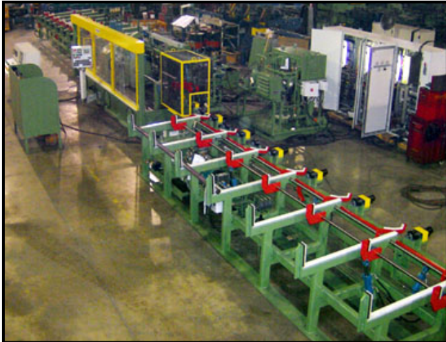
BT3 (75mm) bar turner for peeling niobium-titanium and other exotic metals.
