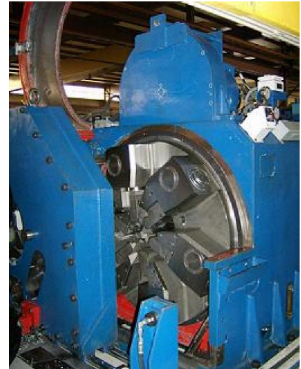
View inside the spindle housing of a new Hetran BT8 - Z large bar peeler recently commissioned by Hetran
